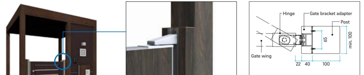
Components for subsequent gate assembly are available as additional accessories. With these, the gate can be mounted directly on posts from a thickness of 100 mm. The design of the gate can be matched to existing roofing and fences.
