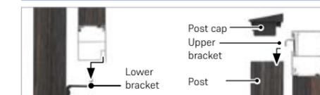
Insert the module into the lower brackets on the post
